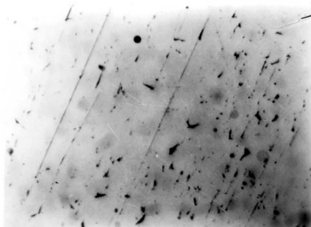
Fig. 6 Optical microphotograph of arc melted vanadium button (unetched).
