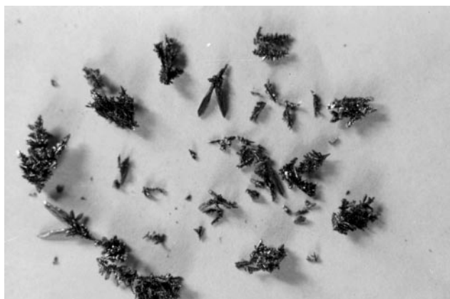
Fig. 5 Coarse and crystalline vanadium fraction ( \geq 840 \mu\text{m} ).
